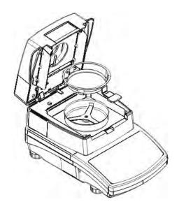
Place the disposable drying pan in its intended holder and place the assembly on the cross-shaped support. support. The display indicates mass of a fitted drying pan.
