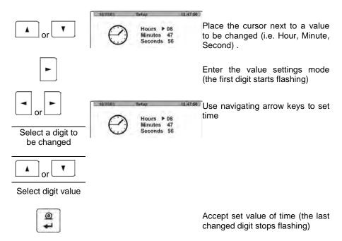
Repeat the process for the following values (minute, second). On setting the new values press **ENTER** key. The moisture analyzer returns to submenu **P3 Date/Time**. The time value visible in the upper bar of the display is changed. After setting the time to a needed value return to the weighing mode following procedure described in point 7.1 of this user manual.
