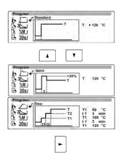
Press UP or DOWN navigating arrow keys to select one of available drying modes: Standard, Quick, Mild or Step.
