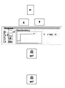
Press right arrow navigating key to change parameter value (the displayed value starts flashing)
