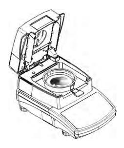
Place a sample to be tested on the drying pan. Mass of a sample should be selected according to previously conducted experiments and features of the tested substance.
