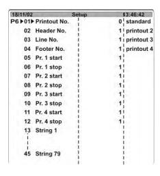
User of a moisture analyzer MAX series can set up to 5 different printout templates which are sent from the instrument to a connected peripheral device (a printer or a computer) through the RS 232 slot.
