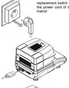
**REMEMBER,** before initiating any activities relates to fuse replacement switch off the moisture analyzer, and make sure the power cord of the moisture analyzer is unplugged from mains!
