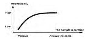
Final measurement result is vastly conditioned by precise and considered sample preparation. A sample used for analysis has to represent the total structure of tested material. Sampling process should determine: sampling means, sample disintegrating, particle size after disintegration, sample uniformity and other. The sampling process should be carried out as quickly as possible, so that a sample does not loose or absorb humidity from surrounding area.
