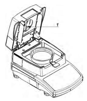
While cleaning make sure not to touch heating filament, as it may damage it.
