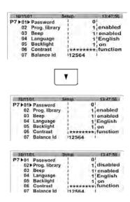
On returning to the main window (with procedure of saving changes) the use can carry out a drying process after setting the basic parameters for drying a sample to be tested. There is no need to select a specific drying program from the database. When setting the parameter Database of drying programs to value 0 – disabled. The user does not have access to the database records saved in the moisture analyzer memory.
