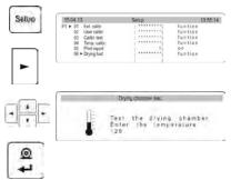
Enter menu group **P1 Adjustment**. Set the marker next to a parameter **06 Drying test**
