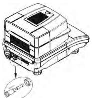
**Tabular fuse ZKT 3.15A T4L 250V** protects moisture analyzer's electric circuits.
