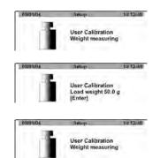
The moisture analyzer gives a command on determining mass of an empty pan, followed by a command to place a weight with pre-determined mass.
