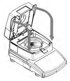
After stabilization of the indication (followed by appearing of a stability pictogram on the display) close the moisture analyzer's lid. The software automatically initiates drying of a tested sample.
