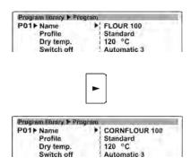
Software structure of the moisture analyzer MAX series enables modifying a parameter which is activated by placed a cursor (black triangle) next to its name (value).
