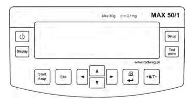
Start Stop **Start/Stop** key – starting / ending drying process according to selected drying mode.
