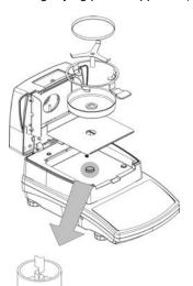
When assembling the pan supporter (bracket) pay special attention to the correct positioning of its mandrel. The mandrel features a cut for its unique positioning against the pan handle, thus preventing their contact and friction.
